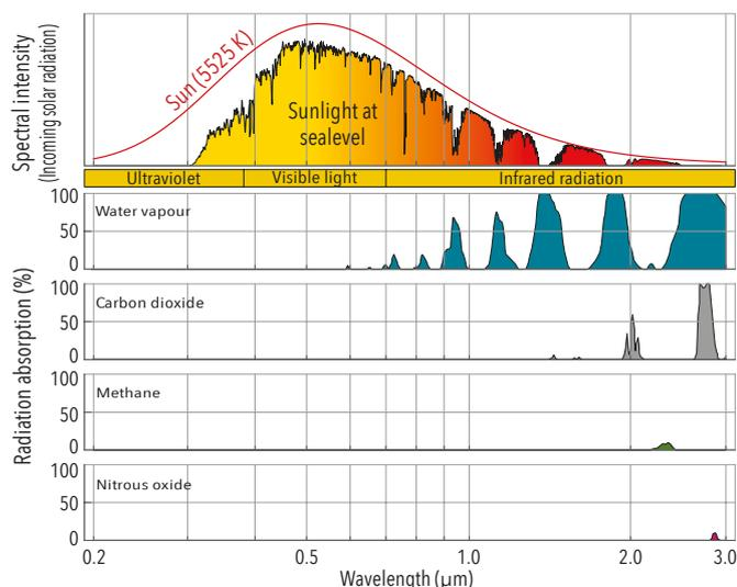
Short wave solar radiation in the 0.2 to 3.0 micrometre wavelength range. The top panel shows the radiation from the Sun at the top of the atmosphere (smooth red curve) while the coloured envelope represents solar radiation transmitted through the atmosphere at sea level. The greenhouse gas absorption peaks (bottom panels) shape the absorption notches in the coloured envelope.
