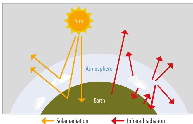
Some of the infrared radiation emitted from the Earth's surface passes through the atmosphere, while some is absorbed and re-emitted back to the surface by greenhouse gases and clouds, making the Earth warmer than otherwise.
