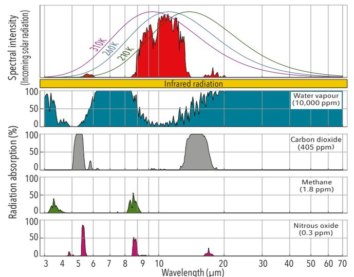
Long-wave IR radiation (smooth curves) that would be re-emitted from Earth in the 3 to 70 micrometre wavelength range at different temperatures - if there were no greenhouse gases. The solid red envelope represents the IR 'spectral window' where IR not absorbed by greenhouse gases escapes to space. The combined spectra of the greenhouse gases (bottom panels) shape this spectral window.
